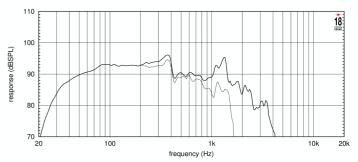
FREQUENCY RESPONSE MADE IN 180 LT. ENCLOSURE TUNED AT 35 Hz IN FREE FIELD (4p) ENVIRONMENT. ENCLOSURE CLOSES THE REAR OF THE DRIVER, THE THIN LINE REPRESENTS 45° OFF AXIS FREQUENCY RESPONSE FREE AIR IMPEDANCE MAGNITUDE CURVE
