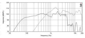
FREQUENCY RESPONSE CURVE MADE ON 125 LT ENCLOSURE TUNED 50HZ IN FREE FIELD (4PI) ENVIRONMENT. ENCLOSURE CLOSES THE REAR OF THE DRIVER. THIN LINE REPRESENTS HIGH FREQUENCY RESPONSE. FREE AIR IMPEDANCE MAGNITUDE CURVE
