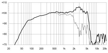
FREQUENCY RESPONSE CURVE OF 12NMB420 MADE ON 18 LIT. ENCLOSURE TUNED 60HZ IN FREE FIELD (4PI) ENVIRONMENT. ENCLOSURE CLOSES THE REAR OF THE DRIVER. THE THIN LINE REPRESENTS 45 DEG. OFF AXIS FREQUENCY RESPONSE
