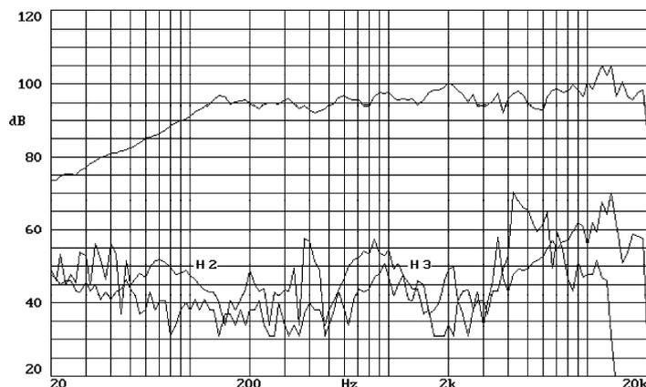
Note: On axis filtered frequency response measured with loudspeaker standing on infinite baffle in anechoic chamber, 1w @ 1m with FD2XA.
