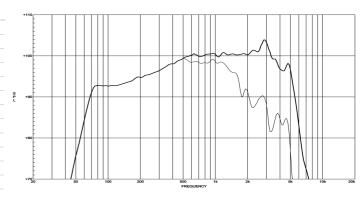
FREQUENCY RESPONSE CURVE OF 10NMB420 MADE ON 30LIT. ENCLOSURE TUNED @ 55HZ IN FREE FIELD (4PI) ENVIRONMENT. ENCLOSURE CLOSES THE REAR OF THE DRIVER. THE THIN LINE REPRESENTS 45 DEG. OFF AXIS FREQUENCY RESPONSE.
