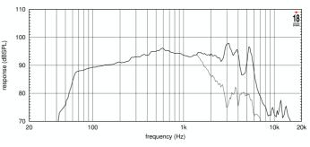
FREQUENCY RESPONSE CURVE OF 8NW650 MADE ON 25LIT. ENCLOSURE TUNED 65HZ IN FREE FIELD (4PI) ENVIRONMENT. ENCLOSURE CLOSES THE REAR OF THE DRIVER. THE THIN LINE REPRESENTS 45 DEG. OFF AXIS FREQUENCY RESPONSE
