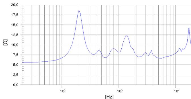
Note: Electrical impedance measured coupled to TD-385 horn
