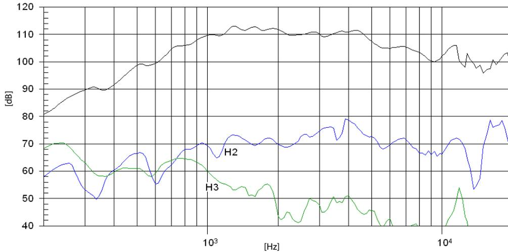
Note: On axis frequency response measured coupled to TD-365 horn in anechoic chamber, 2,83 v @ 1m
