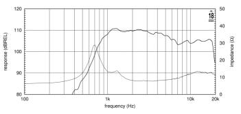
ND 1085 FREQUENCY RESPONSE MEASURED WITH 1W INPUT ON RATED IMPEDANCE AT 1M DISTANCE ON CENTRAL FORWARD AXIS FROM THE MOUTH OF REFERENCE HORN. THIN LINE REPRESENTS IMPEDANCE MEASURED IN SAME CONDITIONS. FREQUENCY RESPONSE CURVE AND IMPEDANCE MAGNITUDE CURVE ON A PLAIN WAVE TUBE
