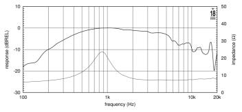
ND 1085 FREQUENCY RESPONSE MEASURED WITH 1W INPUT ON RATED IMPEDANCE ON CENTRAL FORWARD AXIS IN A REFLECTION FREE ENVIRONMENT. THIN LINE REPRESENTS IMPEDANCE MEASURED IN SAME CONDITIONS
