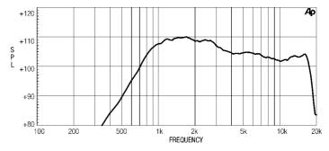
HD1040 MEASURED WITH 1W INPUT ON RATED IMPEDANCE AT 1M DISTANCE ON XT1086 HORN MOUTH AXIS FREE AIR IMPEDANCE MAGNITUDE CURVE
