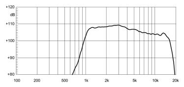
HD125 MEASURED WITH 1W INPUT ON RATED IMPEDANCE AT 1MT DISTANCE ON AXIS FROM THE MOUTH OF HORN XT120 FREE AIR IMPEDANCE MAGNITUDE CURVE
