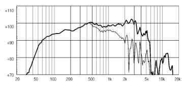
FREQUENCY RESPONSE CURVE OF 12ND930 MADE ON 50 LIT. ENCLOSURE TUNED 60HZ IN FREE FIELD (4PI) ENVIRONMENT. ENCLOSURE CLOSES THE REAR OF THE DRIVER. THE THIN LINE REPRESENTS 45 DEG. OFF AXIS FREQUENCY RESPONSE.
