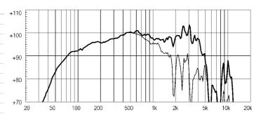
FREQUENCY RESPONSE CURVE OF 12W700 MADE ON 50 LIT. ENCLOSURE TUNED 60HZ IN FREE FIELD (4PI) ENVIRONMENT. ENCLOSURE CLOSES THE REAR OF THE DRIVER. THE THIN LINE REPRESENTS 45 DEG. OFF AXIS FREQUENCY RESPONSE
