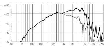
FREQUENCY RESPONSE CURVE OF 10NDA610 (AIC ON) MADE ON 30 LIT. CLOSED ENCLOSURE IN FREE FIELD (4PI) ENVIRONMENT. ENCLOSURE CLOSES THE REAR OF THE DRIVER. THE THIN LINE REPRESENTS 45 DEG. OFF AXIS FREQUENCY RESPONSE.
