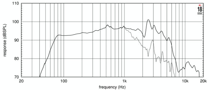
**FREQUENCY RESPONSE CURVE OF 10NW650 MADE ON 25 LIT. ENCLOSURE TUNED @ 65HZ IN FREE FIELD (4PI) ENVIRONMENT. ENCLOSURE CLOSES THE REAR OF THE DRIVER. THE THIN LINE REPRESENTS 45 DEG. OFF AXIS FREQUENCY RESPONSE.**
