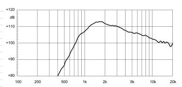
NSD1095N MEASURED WITH 1W INPUT ON RATED IMPEDANCE AT 1M DISTANCE ON XT1086 HORN MOUTH AXIS
