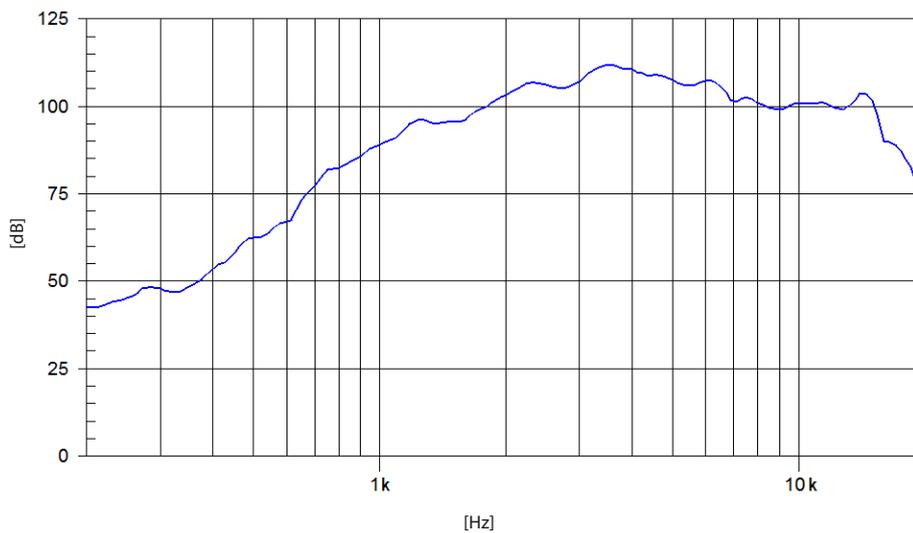
**Note:** On axis frequency response measured couplead to TD-2012/N horn in anechoic chamber, 1W / 1m
